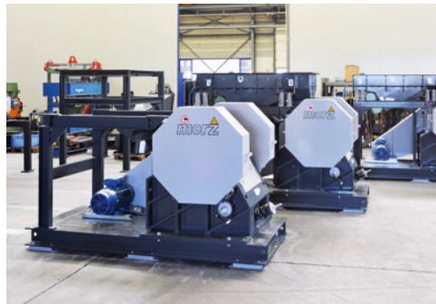
Jaw crusher with vibrating feeder
