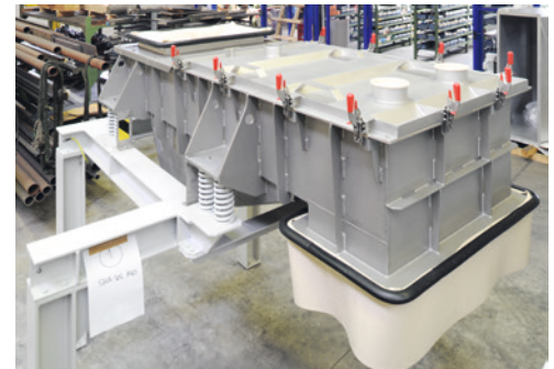
Linear screening machine made in Germany, made by Merz
