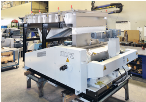
Water-cooled roller mill with electric grinding gap adjustment and vibrating feeder
